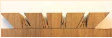
▲ Pic.4 In the meantime I'd been practising my newly invented type of dovetail, the 'SunRay Dovetail'
